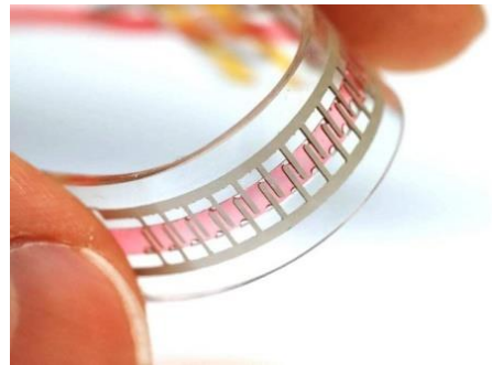
Stretchable pump consisting of soft materials (Credit: Vito Cacucciolo / 2019 EPFL)
