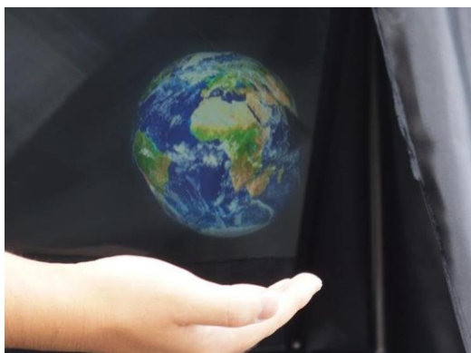
Sunny Day Display. Mid-air image is visible and floats above hand using light from sun.
