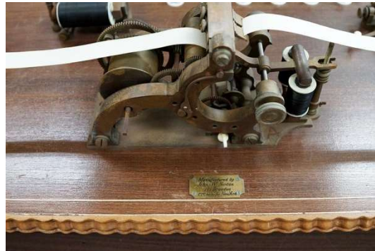
Close-up view of the recording device to emboss Morse code on a strip of paper.
