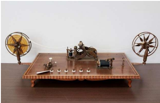
Replica of the Embossing Type Telegraph Key System given as a present by Commodore Perry to the Tokugawa-Bakufu government in 1854.
